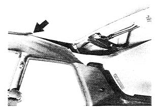
11. Remove mounting screws of element guides and transfer gearbox.
