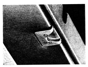
6. Cable anchors located in the lifting roof lid must be adjusted that the cable of the lifting roof runs parallel to the cable of the car roof.
