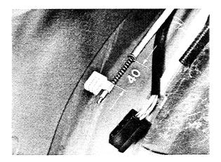
6. Work drive with raising cable into guide rail of electric drive, route along the rail and clip on counterpiece in cam.
