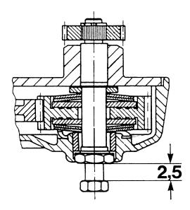
To guarantee perfect operation of the slip clutch, the adjustment should be made by measuring the power input of the sun roof motor.
