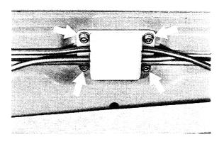
Bolt rear end of element guides on roof hoopsticks (without tension).
