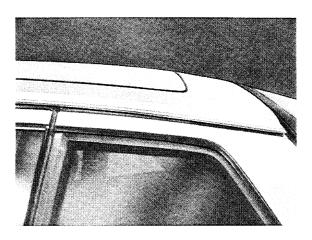
2. Remove roof and pull off edge guard, cement roof liner on body and slide on edge guard. Screw trim panel on roof frame and install caps on heads of screws. 3. If staybolts of element guides are not in neutral position + 3 mm (see sketch), left trim panel must be removed in luggage compartment and excessive deviation eliminated by adjusting the switch lever on the rail.
