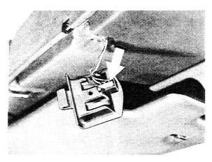
2. Unscrew lifting roof mount and press out of wind deflector.
