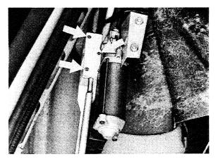
Connect plugs. Place holder on end of rail on studs of tailgate and screw on nuts.
