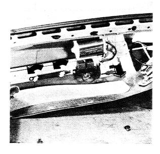
3. Unscrew and remove adjusting screw (a) with the wrench.
