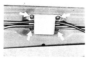
12. Remove assembly set from car by pulling long pipe out of C pillar.
