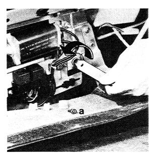
5. Screw in adjusting screw (a) again and adjust the slip clutch (see page 61 - 18).
