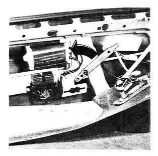
4. Turn the now visible threaded sleeve anticlockwise with the wrench until the roof is closed.
