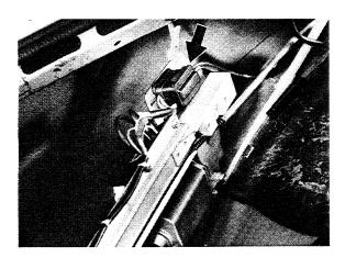
10. Engage console of electric drive in rear frame profile, screw on nuts and plug console claws on edge guard. Tighten all nuts.
